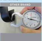
Uneven thickness between 2.0-~3.5mm, higher risk of leakage due to constant pressure attack at the thinnest area
