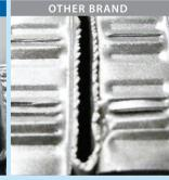
Insufficient and poorly cut louvers
